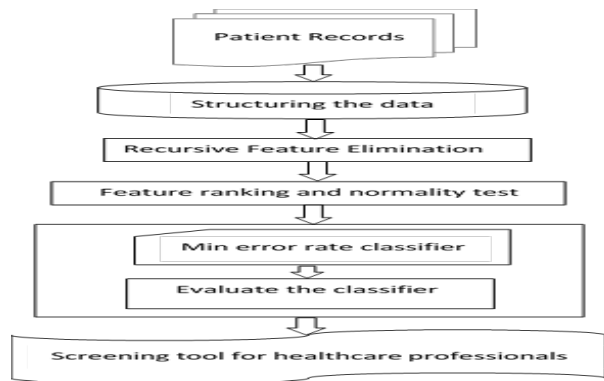
Fig. 1: High level diagram of the smart screening tool for LBW prediction
